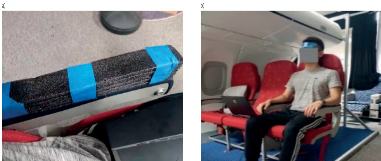
Figure 2. Experimental protocol schematic in the study on the relationship between seat armrest height and human neck comfort when using a smartphone while sitting on a passenger seat during the flight: a) seat armrest height increased by 5 cm and b) wireless Inertial Measurement Unit Sensors (IMU) placed on the forehead
