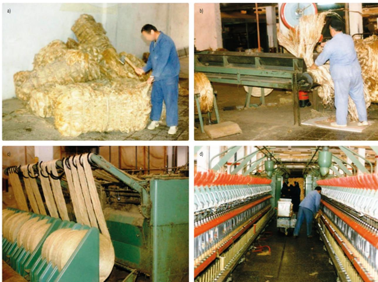
**Photo 1.** Dusty sections of the factory: a) opening and spreading, b) softening, c) carding, d) spinning
