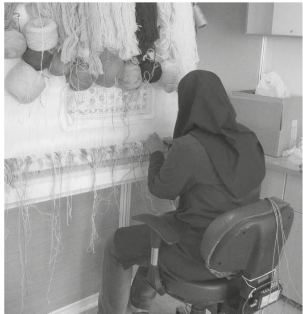
Photo 2. Workstation B: a high vertical loom and a weaver sitting on the chair with backrest and armrest
