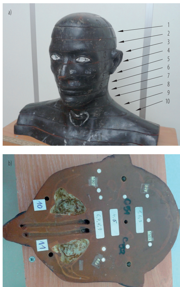
Photo 1. Anthropomorphic Rando phantom: a) marked successive slices, b) a single slice with marked holes where thermoluminescent detectors (TLD) were inserted
