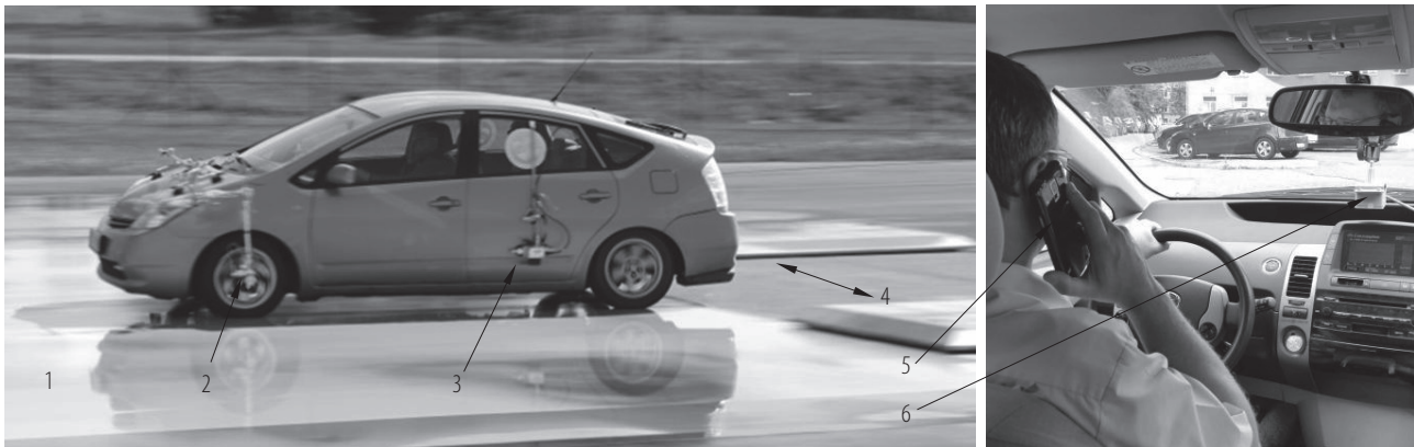
1 – slip pavement; 2 – steering angle sensor; 3 – speed and sideslip angle sensor; 4 – moving plate; 5 – phone cell; 6 – body yaw rate sensor.
