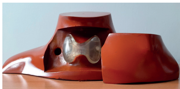
Figure 2. Radiology Support Devices (RSD) neck phantom with thyroid gland
