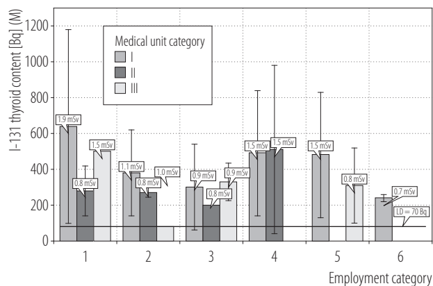
Figure 4. Average thyroid content of radioiodine (I-131) and effective dose for employees in medical units during measurement carried out in 25 hospital units in Poland Employment category: 1 – electro-radiologist, technician, 2 – medical physicist or a radiological protection inspector, 3 – medical doctor, 4 – nurse, 5 – cleaner or orderly, 6 – radio-immunologist, radiochemist, conservator engineer. For categories of medical unit explanation, please see Table 1.
