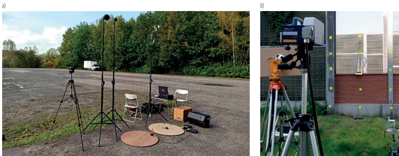
Figure 1. Measurement setups for studies in the field of a) acoustics and b) vibrations, Upper Silesia, Poland, 2024
